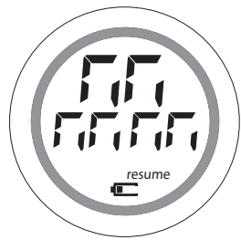
test pattern 2 (alternate segments activated)
