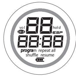
test pattern 2 (alternate segments activated)
